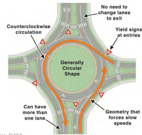
Figure 71: Illustration of Roundabout Element
