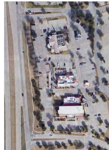
Figure 72: Driveway Consolidation in Frisco, TX
